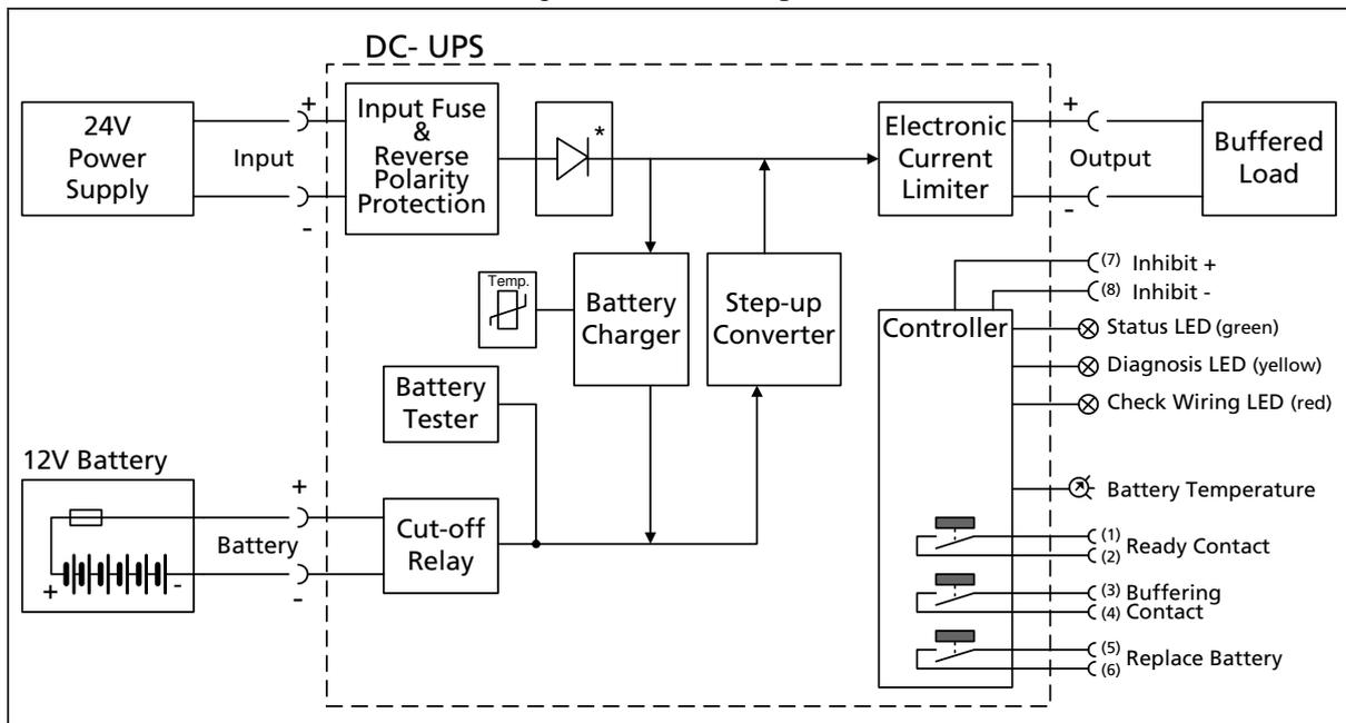
\*) Return current protection; This feature utilizes a Mosfet instead of a diode in order to minimize the voltage drop and power losses.
